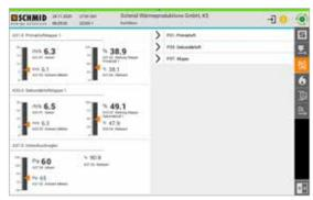
The dashboard gives the operator an overview of the current system status at any time. The desired information on the dashboard can be selected individually. The new operating system is divided into two areas. The first menu group is explicitly for the operator and includes all system information that can be important on a daily basis.
